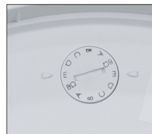
120W Transformer: The transformer has a front tap selector switch protected behind the press-fit grille.
