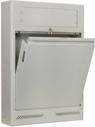
Wall-mount rack with two bays. Remove the top panel to utilize the 3U upper bay. The lower (main) bay tilts down when opening to operation or service position.
