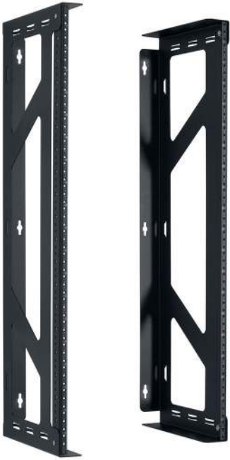
The two-part VWR mounts on 16" or 20" centers to accommodate 19"W or 23"W equipment.
