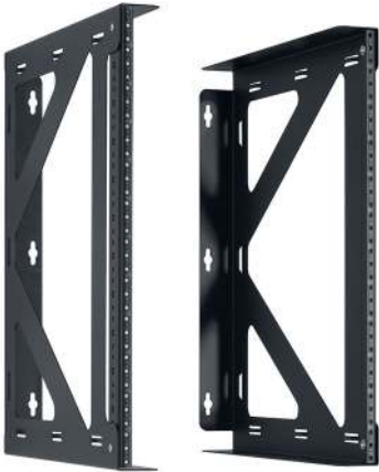
The two-part VWR mounts on 16" or 20" centers to accommodate 19"W or 23"W equipment.
