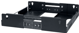
Changing project specs are no problem—with the Vari-Rack's adjustable top and base you don't actually set rack depth until assembly. Corner post mounting rails are also ready for last minute changes with printed cut marks to guide in-the-field trim to height.
